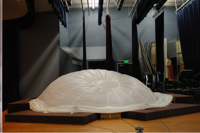
Inflating the dome, notice bottom of dome is taped down.
